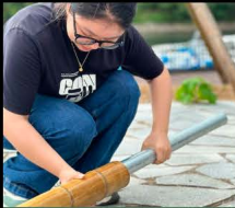
Use steel bars to pierce the bamboo for subsequent use
